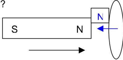
Because of Lenz's law the conductor develops a current in a direction to oppose the change in magnetic flux. So in this case the induced current produces a magnetic field opposite to the magnet (N pointing to the left). This causes the loop to be repelled by the magnet.
