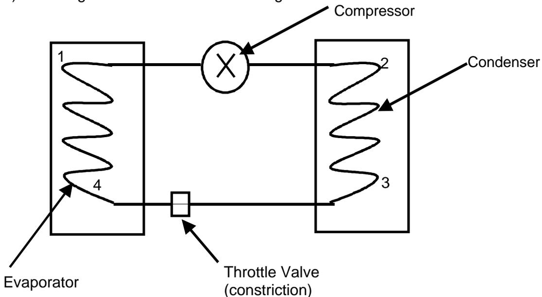
For each of the four marked locations (1-4) answer in the chart below whether: the fluid is a liquid or gas; the fluid is hot, warm, cool or cold; heat is flowing into or out of the fluid; the fluid is at high or low pressure and finally is the location inside or outside the house. (Each answer is worth 1 point).
