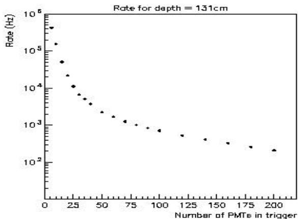
Figure 4 Trigger rate vs # of PMTs hit.
