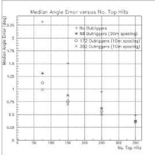
**Figure 7 - Median angle error versus number of hits in the top layer for different outrigger arrangements**
