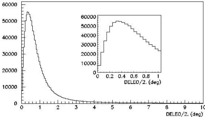
**Figure 6 Distribution of "DELEO/2" for Milagro. The intrinsic angular resolution of the shower fit is giving by the peak of this distribution. This indicates that Milagro's intrinsic angular resolution is approximately 0.35 degrees.**
